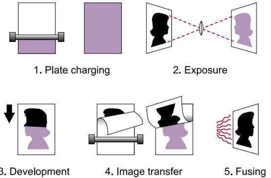
**How xerography works: A specially prepared plate is charged with static electricity (purple). The charge drains away wherever light hits the plate; dark areas remain charged. A black powder of opposite charge will stick only to those areas, and when a piece of paper is pressed against the plate the powder (and the image) is transferred. Heat treatment binds the powder to the paper.**
